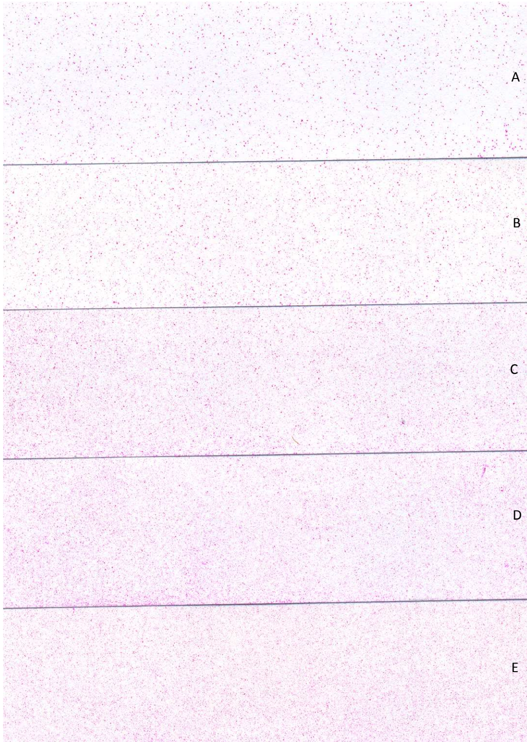
Plate 1. Droplet distribution pattern for 1.2 mm nozzle opening at different speeds (A) 2000,rev/min (B) 3000,rev/min (C) 4000, rev/min (D) 5000, rev/min (E) 6000 rev/min.
